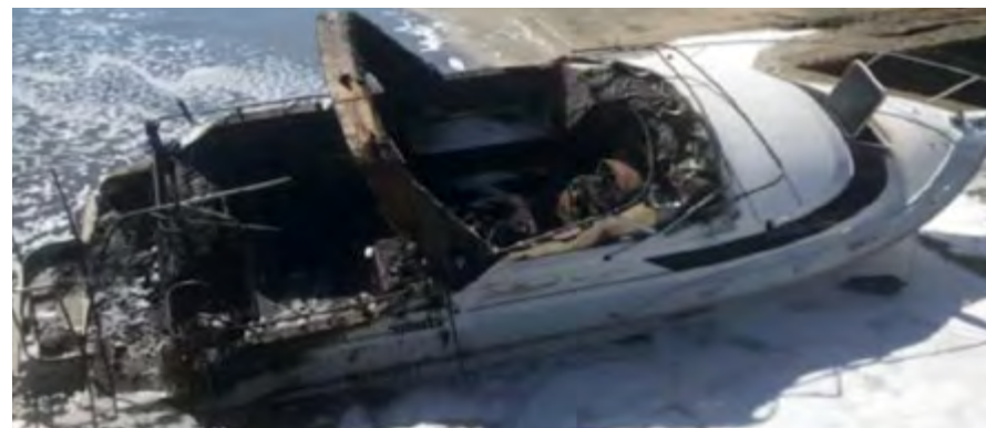
A vessel burnt to the gunwale. The forensic investigation identified the fire as likely to have resulted from leaking fuel lines. Reinforced rubber fuel lines are considered to have a service life of 10 years. The burnt vessel is 25-years-old and should ideally be on its third set of replacement fuel hoses. Without a maintenance log, how can we know? By the time visual inspection determines a fuel hose is brittle and is delaminating, the risk of failure is imminent.
