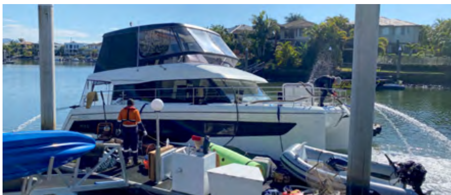
A power boat that is partially sunk due to an exhaust hose being incorrectly fitted.
