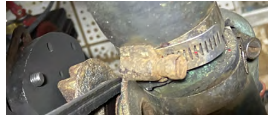
A bulging cooling hose with a very corroded hose clamp well past its replacement date. Should the hose fail, the engine cooling system may fail and engine damage occur, resulting in a loss of power. A maintenance plan to inspect and replace could ensure that these items are in better condition.
