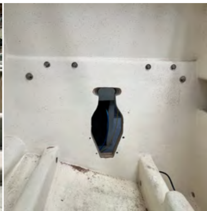
Asahi II - Inspecting prior to engine and sternleg fitting
