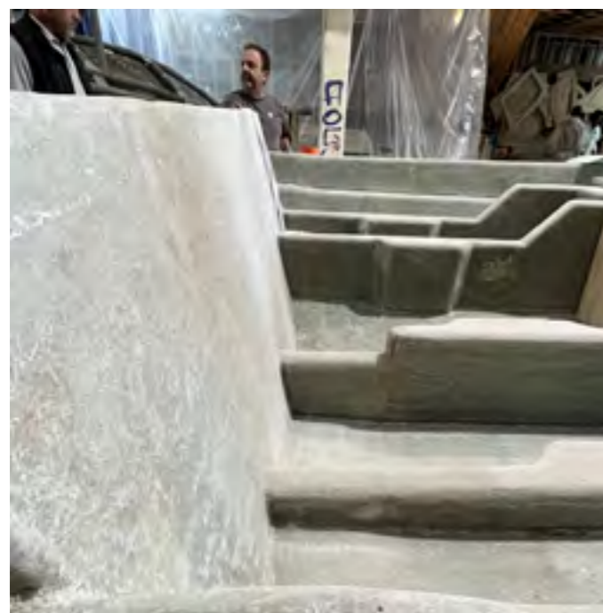
Asahi II Inspection Visit 1 - Layup of the hull
